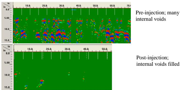
Fig. 5 Sample radar traces showing internal masonry wall condition before injection (top) with many internal voids as indicated by multiple reflections within the radar trace. Following injection the radar trace shows the wall to be essentially solid (bottom) with no significant reflections.
