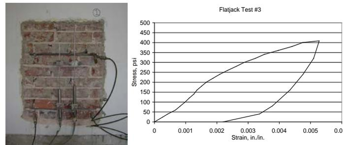
Fig. 3 Masonry deformability test conducted using the flatjack method. Test setup shown at left; at right is a typical stress-strain curve. Masonry compressive strength was measured to be in the range of 450 psi.
