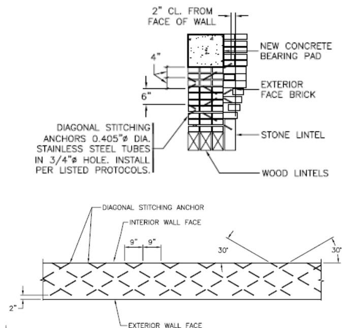
Fig. 4 Design detail showing diagonal stitching installed as confinement reinforcement: wall section (top) and horizontal plan section (bottom). Stainless steel tubes inserted into drilled holes were injected with CIF to bond new reinforcement to surrounding masonry.
